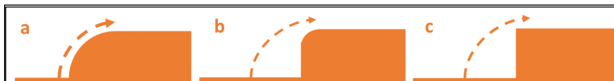
Figure 2. Obstacle modifications: (a) rounded obstacle, (b) rounded edge obstacle, (c) squared edge obstacle.
