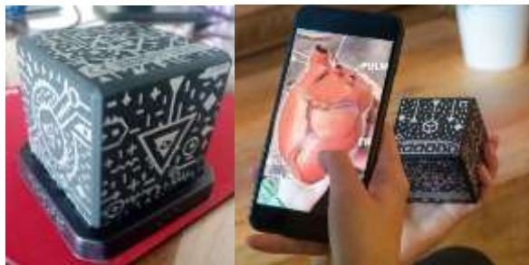
Figure 2. Marge Cube , an example of augmented reality for educational purposes. Through a dashboard, it is possible to upload .fbx, .obj, .stl, .gltf files for manipulation using the cube.
